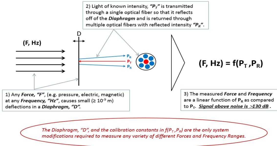
**Figure 1 – Basic Principles of Intensity Modulated Optical Sensing**
