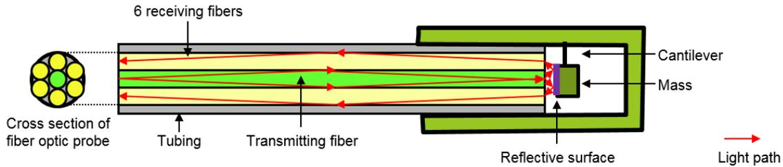
As the accelerometer vibrates, the cantilever bends due to the inertia of the mass, and the mass is displaced relative to the fiber optic probe. Acceleration is calculated based on the displacement of the mass and frequency of its vibration based on the following relationships:
